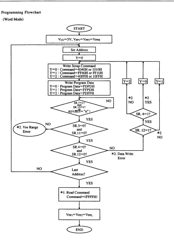
Note) \*1. Write FFFFH after the last block write operation to reset the device to Read Array Mode.
