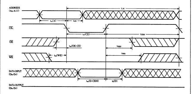
Note: 1. To write attribute memory,  $\overline{REG}$ ="LOW" and either  $\overline{CE}_2$ ="LOW" or else  $\overline{CE}_2$ ="HIGH" and  $A_0$ = "LOW"
