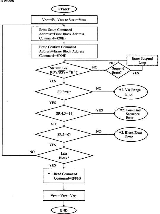
Note) \* 1. Write FFH after the last block erase operation to reset the device to Read Array Mode.
