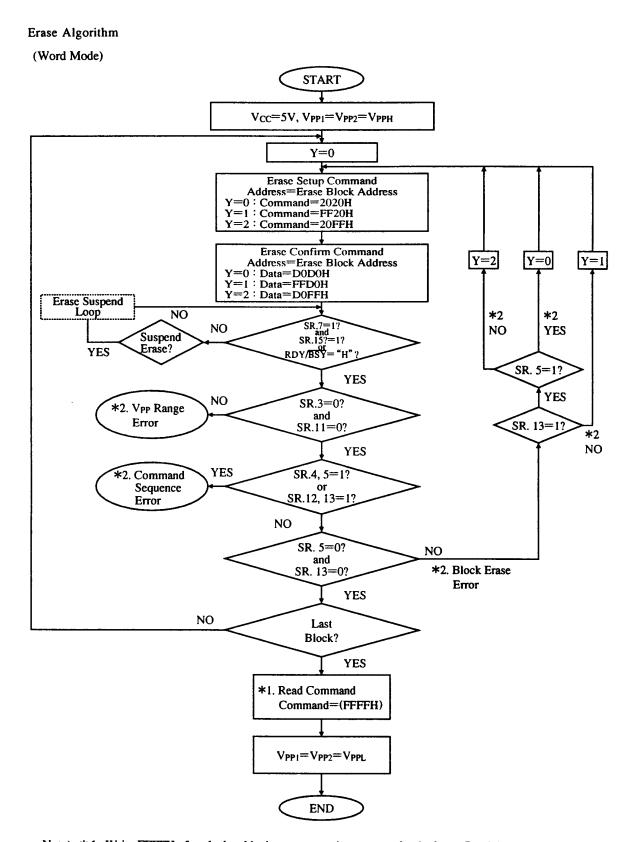
Note) \* 1. Write FFFFH after the last block erase operation to reset the device to Read Array Mode.
