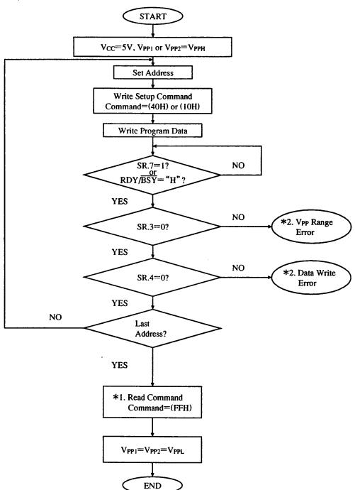
Note) \* 1. Write FFH after the last block write operation to reset the device to Read Array Mode.
